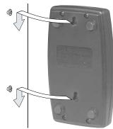
**Note:** Do not mount the amplifier on any other electronic device. Stacking components may cause overheating.
